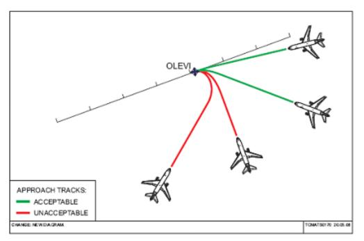
Figure 4: Radar Vectors to RNAV Approach
