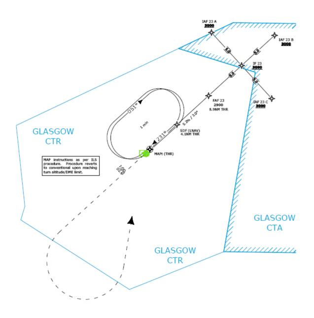
Figure 1: Glasgow RWY23 LPV procedure
